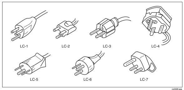
Figure 4. Line Power Cord Types Available from Fluke
