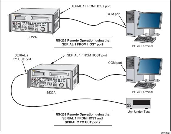
Figure 2. RS-232 Remote Connections
